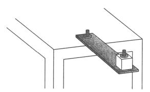
Mech. 1. A thin, flexible metal plate attached at one end to a platform, as shown above, can be used to measure mass. When the free end of the plate is pulled down and released, it vibrates in simple harmonic motion with a period that depends on the mass attached to the plate. To calibrate the force constant, objects of known mass are attached to the plate and the plate is vibrated, obtaining the data shown below.
