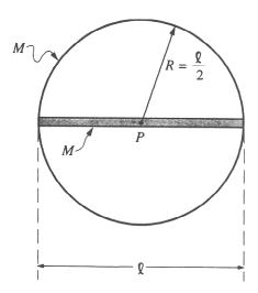
The rod is now glued to a thin hoop of mass M and radius  $R = \ell/2$  to form a rigid assembly, as shown above. The centers of the rod and the hoop coincide at point P. The assembly is mounted on a horizontal axle through point P and perpendicular to the page.
